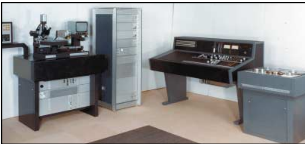
Neumann disc mastering system: VMS80 lathe; SX74 cutterhead; SP79 console; SAL74 cutter logic drive; and MT80 preview tape deck.
