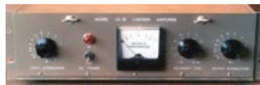
The main difference in the CCA LA-1D is the use of a 12BH7 valve for the output stage. It also offers greater release time flexibility by using two switchable time stages.
