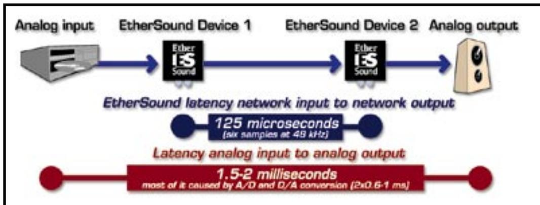
chain, star, or a combination of both. The extended technology specification mentioned above, which enables bi-directional audio-distribution, has further improved system flexibility. Before the release, the EtherSound protocol was restricted to unidirectional audio distribution.
