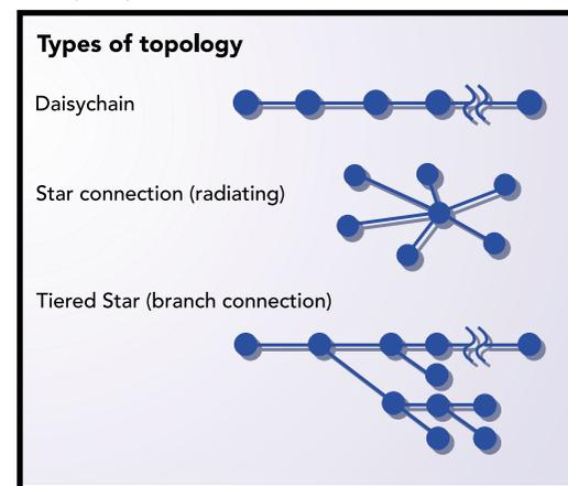
The distance between any two nodes is determined by a combination of the cable length and the number of hops. The standard 1394 copper cable length is normally up to 4.5m and the maximum number of hops between any two nodes is 16, resulting in a maximum distance of 72m between nodes. This is often fine for small to medium-sized studio installations, but for applications that require longer distances, 1394-compatible fibre optic interfaces and long haul repeaters can be employed.
