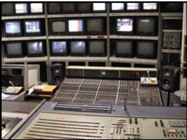
the demands, including an orchestra, singers, groups and audience. The chosen console has 32 faders, 182 inputs with optical cables running the 100m to the studio floor with a choice of four wall boxes patched according to the project in hand, and replaced an old Tesla console.
