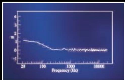
Fig. 7. Acoustic source plot for a 700 litre, wide-range, flush-mounted, studio monitor system. Note how the NS10M's response (Figure 5a) mimics that of this large monitor system.
