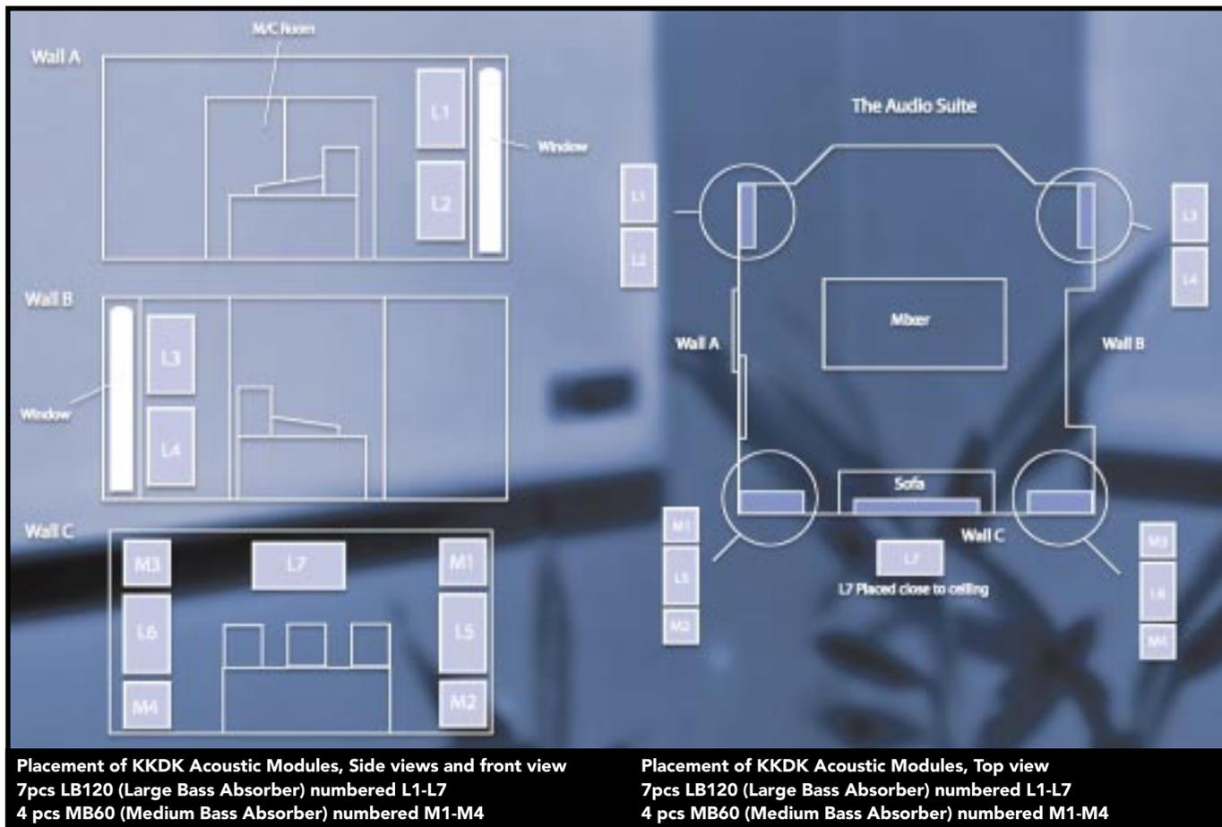
Placement of KKDK Acoustic Modules, Side views and front view
