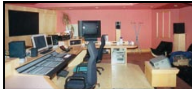
Fig. 3. Stereo control room adapted for surround in the general manner shown in Fig. 1. The surround loudspeakers are mounted on pedestals at the sides and rear of the room [Eurosonic, Madrid. Control room designed by Sam Toyashima].
