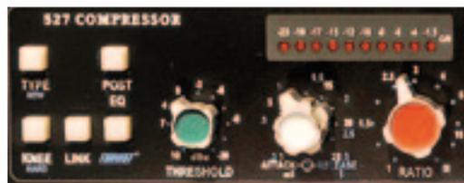
Knobs are provided for Threshold, Ratio, and a dual-concentric Attack and Release. And there is also a Post EQ button that swaps the two sections round in processing order. With all the different possibilities here, the compressor can satisfy most
