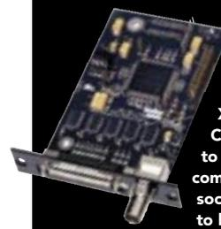
The X-HD option card allows direct connectivity between Pro Tools|HD systems and the X series units. The X-FireWire Card enables direct connection to any FireWire-equipped computer. Two FireWire 400 sockets allow further X-Series units to be daisy-chained from a single PC or Mac connection.
