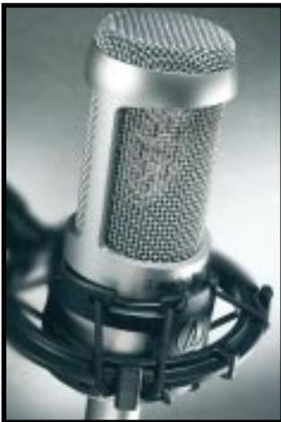
less than the non-valve AT4050. What is clear is that this is purely for the amplifier, as the capsule is actually a large-diaphragm back-electret design, offering a fixed cardioid response.
