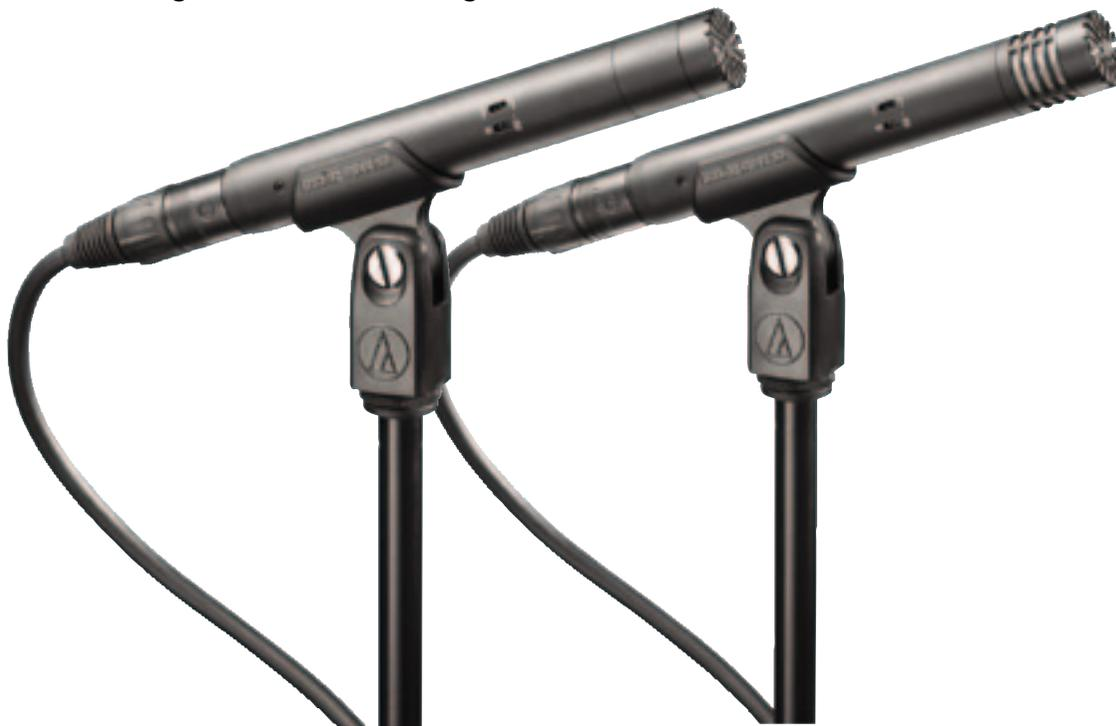
The Audio-Technica 4021 and 4022 are relatively recent additions to the company's 40 series product range. While there are existing small diaphragm capacitors in the range, the key difference here is that the capsule is a back-electret design rather than externally polarised. The 4021 has a fixed cardioid response, while the 4022 is omnidirectional. Other than the ports on the side of the cardioid microphone, they are pretty much identical visually.
