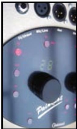
clue as to the integrity of the audio circuitry here — nearly every function is switched by gas filled relays — even the gains, which step through relays in dB steps. Not only does this approach keep audio paths as clean as possible, it also means that every control input on the device itself is 'soft', which in turn means that remote control of the device is easily achieved — more on this later.
