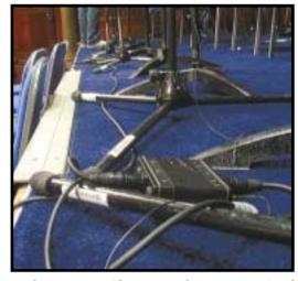
to the rescue. With some rather unconventional mounting arrangements (4061 microphones attached to miniature clips mounted with sticky pads to the spigots of some small stands), a pair of 4061s was assigned to each of the first and second flutes, oboes, clarinets and bassoons. Level and pan was set for each microphone, and the summed output happily fed the last two tracks on the recorder.
