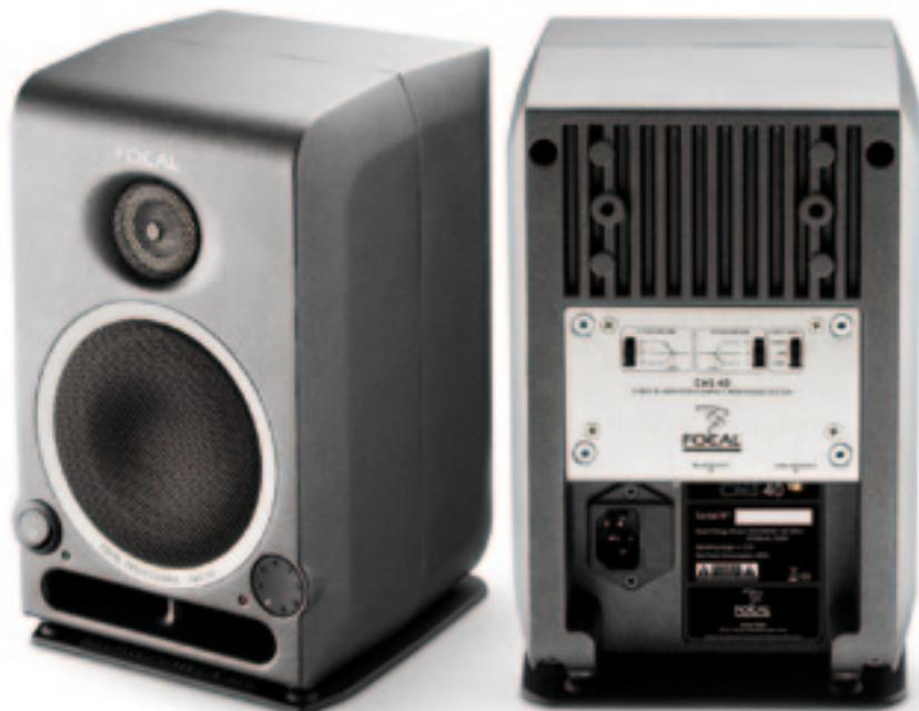
The CMS 40 is the smallest speaker in Focal's range of studio monitors, with overall dimensions of only 238mm high by 156mm wide by 155mm deep. It is a two-way active speaker comprising a 4-inch woofer with a Polyglass cone and a 25mm aluminium/magnesium inverted dome tweeter. The power amplifier, crossover and protection electronics are all built-in to the cabinet which is made of cast aluminium. The speaker is supplied
