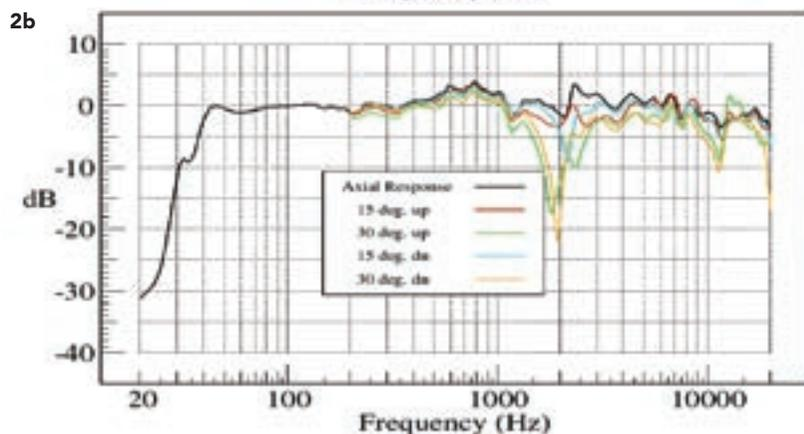
**Figure 2a, 2b. Off-Axis Responses.** These demonstrate the ability of the loudspeaker to radiate effectively at other angles other than on-axis. Problems such as excessive beaming, side lobes and interference between the outputs of separate drivers are highlighted by these plots.
