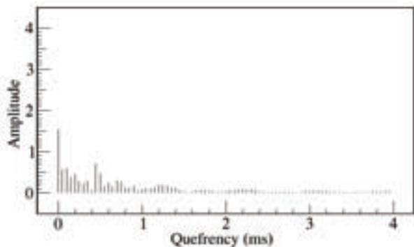
**Figure 5. Power Cepstrum.** A diagnostic Measure. Used to assist in finding the cause of frequency response unevenness. Distinct echoes and other reflections, such as diffraction from cabinet edges, show up as spikes in the power cepstrum.
