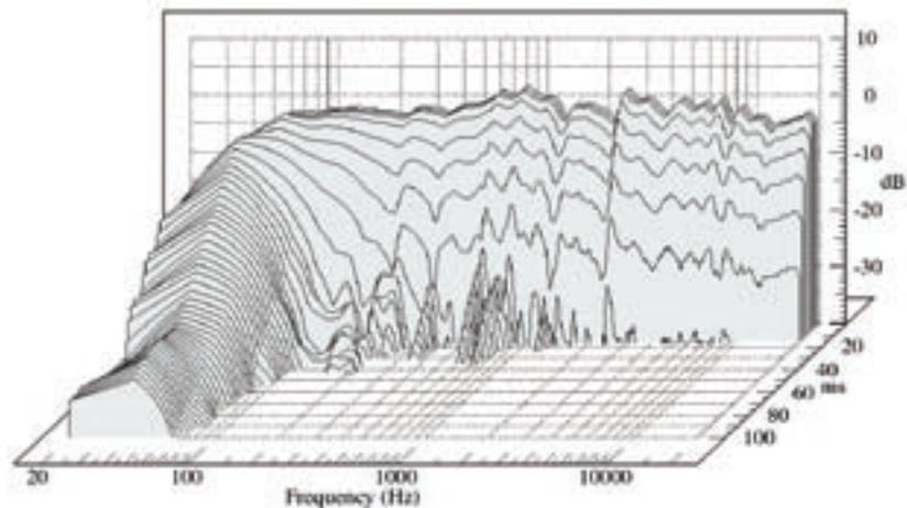
**Figure 6. Waterfall Plot.** A combined frequency response/time response plot. This shows the time taken for frequency components of the signal to decay to a low level when the signal is stopped. Resonances and some other phase-related problems show up as extended decay times. This is particularly revealing of low-frequency roll-off related ringing.
