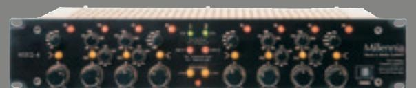
It features the 'World's first and only' all-discrete, true differential Class-A input buffer/amplifier, selectable balanced or unbalanced input, a 'greatly improved' 3rd generation FSA-03 all-discrete EQ amplifier, an improved output stage, no muting required (as with Twin Topology), true hard-wire bypass when EQ is not selected, and an upgraded power supply.
