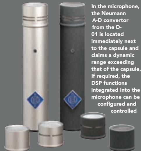
In the microphone, the Neumann A-D converter from the D-01 is located immediately next to the capsule and claims a dynamic range exceeding that of the capsule. If required, the DSP functions integrated into the microphone can be configured and controlled
