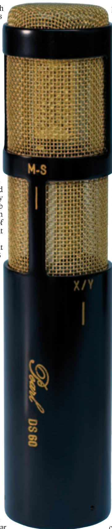
pattern that moves from omni, to cardioid, to fig-8 and anything in between. But remembering that the capsules are oriented 90 degrees apart also means that taking the output of one diaphragm on the bottom capsule, and another from the top capsule enables XY stereo recording. Or mixing both capsules to fig-8 makes an instant Blumlein pair. Or mixing one capsule fig-8 and one cardioid/omni gives you MS. Or... well, you get the idea.
