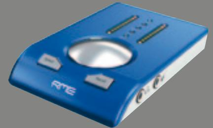
It employs RME's SteadyClock and the digitally controlled preamps have individually switchable 48V phantom power. The feature set includes optical I-O, usable as ADAT port with SMUX support or SPDIF for sessions at up to 192kHz. In combination with an ADAT converter, like the RME ADI-8 DS/QS or OctaMic II, the Babyface provides 10 analogue input and 12 output channels. A headphone output is available directly on the unit and also on the breakout cable.
