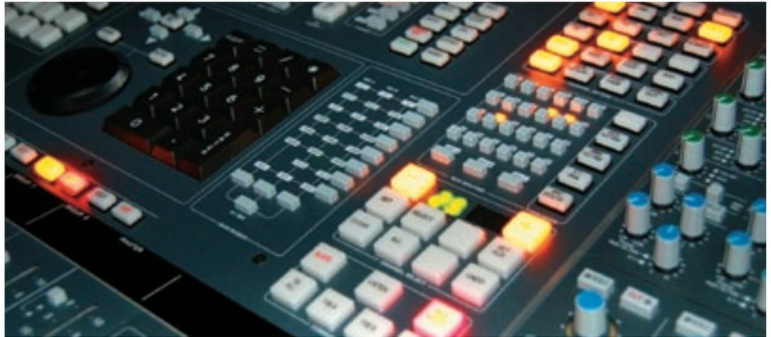
Multiple TFT screens offer a lot more information than a conventional meterbridge with automation fader position, analogue level and workstation level. Processing assignment in each of the two paths is also shown. When it comes to resetting the console, each screen can be paged through the settings for each of its six associated channel strips. Therefore multi-operator Total Recall becomes possible, speeding up the process to the point where it is almost painless. Total Recall on steroids.
