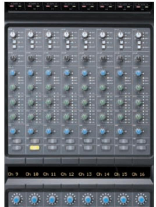
Matrix is most likely to be used in this manner. The first channel input will take the output of a mic pre, an instrument or DI box. The second input takes the return from the DAW. The Channel direct output, CHOP, will normally feed the pre-fader signal to a DAW track. When overdubbing there is an automatic switching mode, Auto Mon, which will switch between
