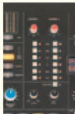
The small section at the top centre of the console provides basic monitoring function and mic preamp operation. Monitoring comprises a volume knob to control stereo DAW level as it passes through to the monitor outputs. However, there is more. The mic preamps' signals can be blended with the mix for zero-latency monitoring while their direct outputs are recorded. A Blend knob balances the preamps with the mix.
