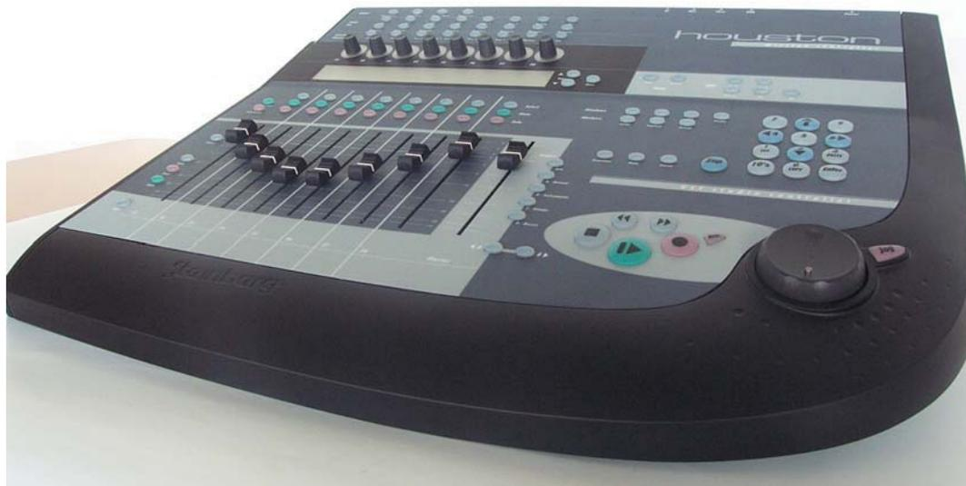
nels as you may have in a VST mixer. Two keys shift the physical strips along the virtual VST mixer eight channels at a time or, used with the Shift key, one channel at a time. The VST mixer can be re-arranged to put specific channels together 'in view' by creating fader sets, invoked with the Fader Sets key and the numeric keypad. Other keys adjacent to the master fader allow more direct access to 'normal' channels, instrument channels, groups and busses.
