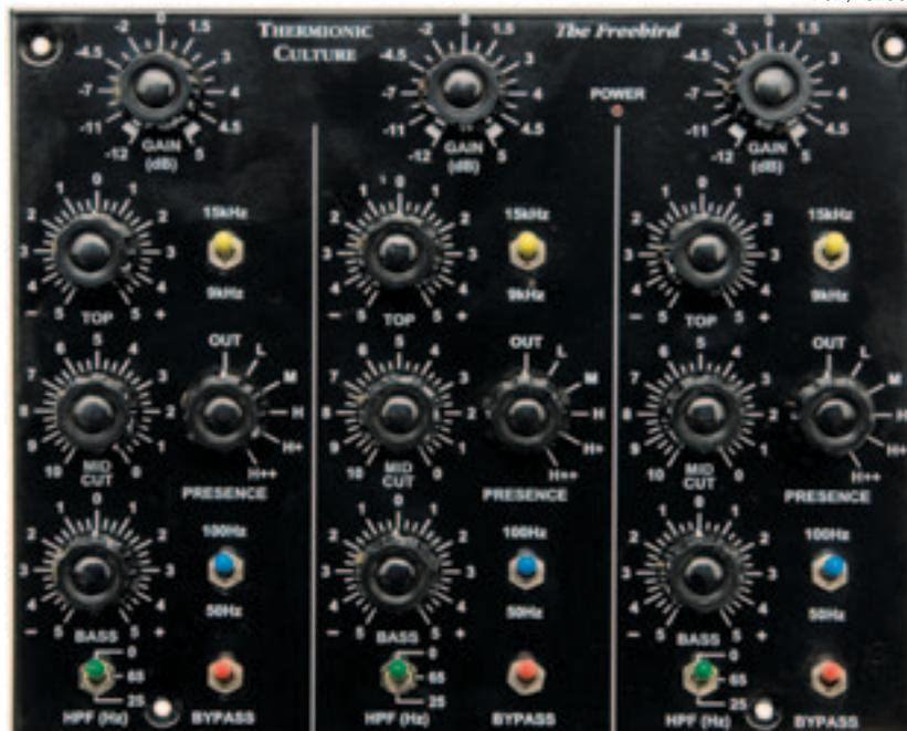
15kHz and 9kHz. The knob is legended from -5 to +5 with zero at the centre (top), which doesn't sound like an especially generous range. However, the actual scope is -16dB to +14dB. The 9kHz setting adds rich treble, and 15kHz is particularly silky; usually +2 on the legending is plenty for general enhancement, although full boost is useable and never nasty.
