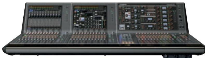
The central component of the RIVAGE PM7 system is the CSD-R7 digital mixing console. The same size as RIVAGE PM10's control surface, the CSD-R7 has the DSP engine built in. Featuring 120 input channels, 60 mix buses, 24 matrices and a comprehensive selection of 48 top-quality plug-ins, RIVAGE PM7 also provides a similar mixing capacity to RIVAGE PM10.
