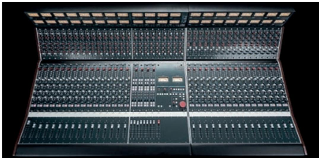
say eliminate crossover distortion entirely. These new op-amp cards offer extended headroom, dynamic range, and frequency response while generating exceptionally low noise and distortion. Custom-designed transformers are also included on every single input and output of the 5088, electrically isolating the console with a true floating ground while also imparting the sound quality of his classic designs.
