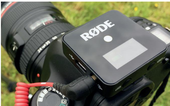
/ The Wireless Go receiver belt-clip doubles as a camera hot-shoe mount
