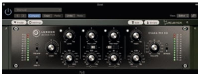
London describe the four-band parametric Osaka as "somewhat Oxford-esque in inspiration", although when using the mid-bands on the highest Q setting on toms I found myself reminded of a Trident TSM console (only less noisy of course). Each of the four EQ sections are individually activated by clicking a little button to the left of the boost/cut knob. Despite a bit of latency in using them, it's convenient to be able to punch the sections in and out.
